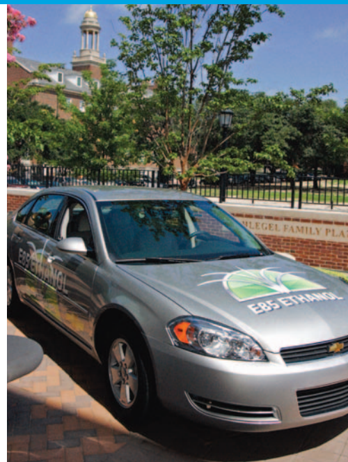
Flexible fuel vehicles can be fueled with unleaded gasoline, E85, or any combination of the two.
